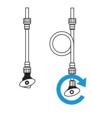
1 Turn off cold water supply under the sink.
