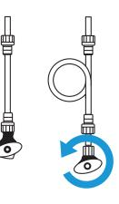
2 Remove the old cartridge from the manifold by rotating it to the left until it unlocks. Pull cartridge down and discard.
