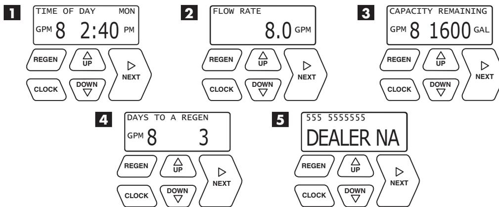
If the system has called for a regeneration that will occur at the preset time of regeneration, the words "REGEN TODAY" will appear on the display. If a water meter is installed, "GPM" flashes on the display when water is being treated, indicating gallons per minute flowing through the system.
