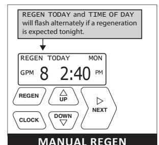
Once a manual regeneration is initiated, the unit will enter the first regeneration cycle position. Once the unit advances to its first position and subsequent positions thereafter, (see Start Up Instructions for regeneration sequence) the water filter will deliver water, but it will be untreated.
