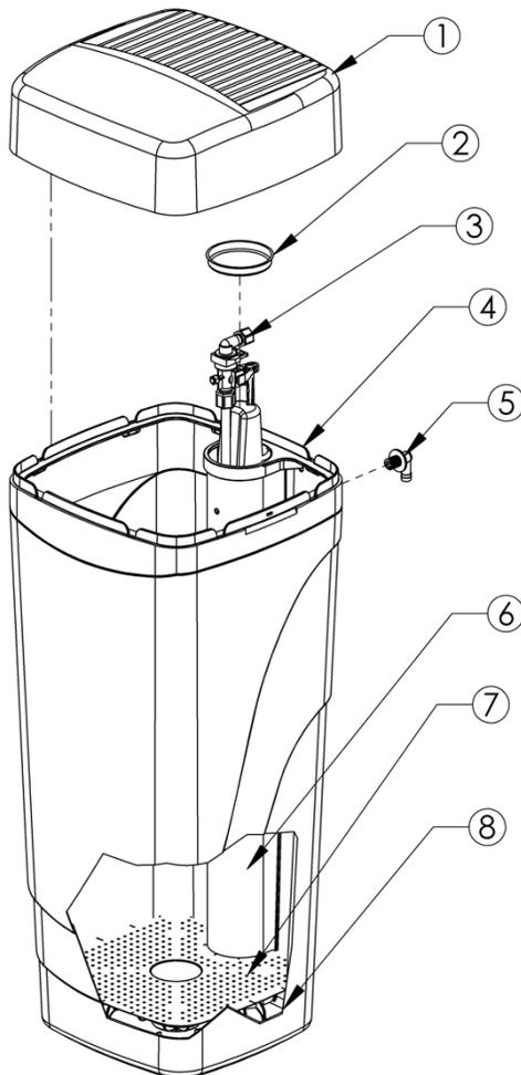
**Figure 10: Standard Brine Tank Assembly (25, 25CX, 35, and 48)**
