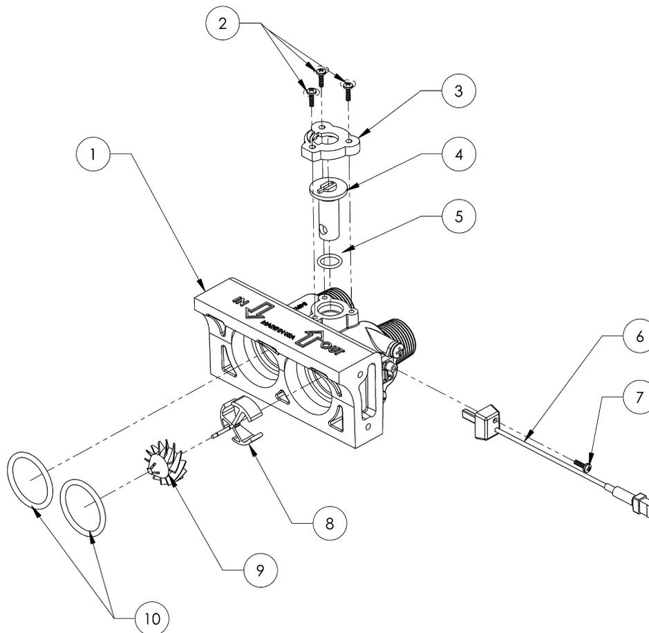
**Figure 21: 3/4-inch I/O Adapter Assembly with Blending Valve**
