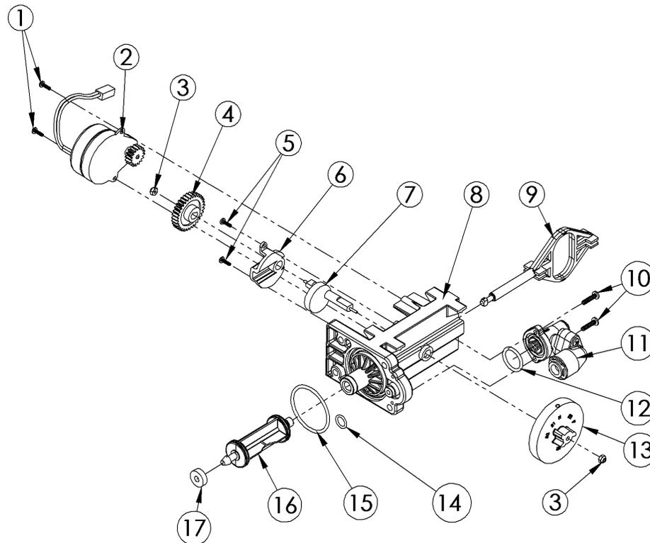
Figure 18: Drive End Cap Assembly
