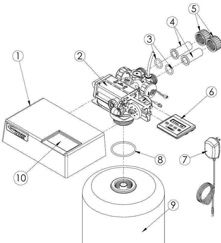
Figure 8: Hook-Up/Cover Assembly
