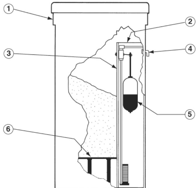
**Figure 11: Standard 24" x 50" Brine Tank (64 and 105)**
