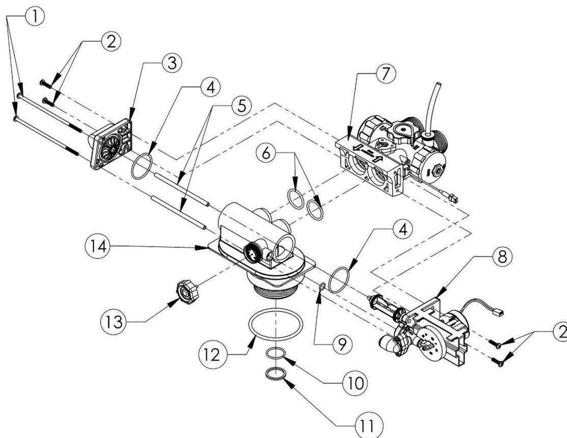
Figure 15: Valve Assembly
