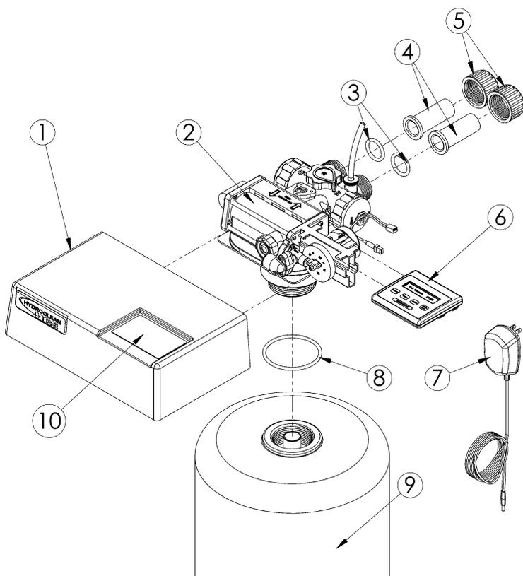
Figure 8: Hook-Up/Cover Assembly
