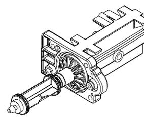
Rotate The Piston Assembly 90 Degrees
