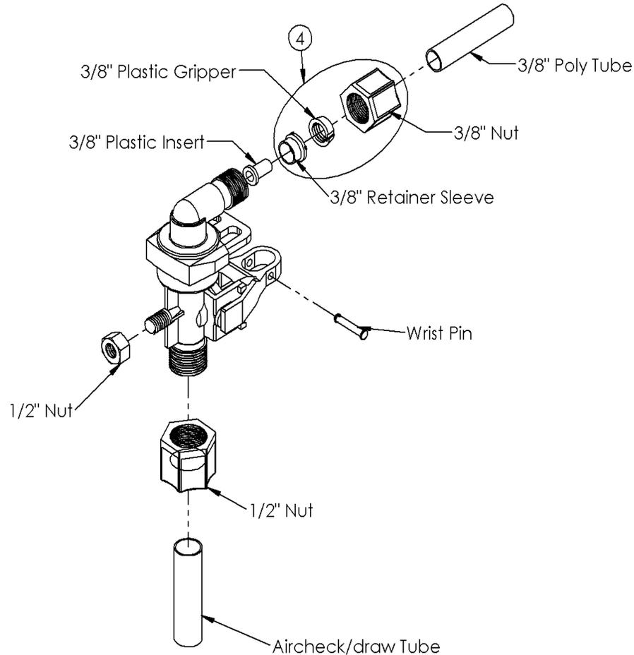
**Figure 23: Brine Valve Elbow Installation**
