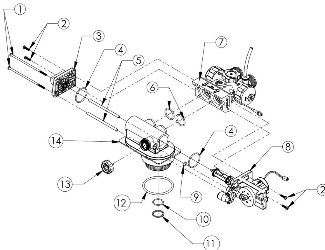
Figure 15: Valve Assembly
