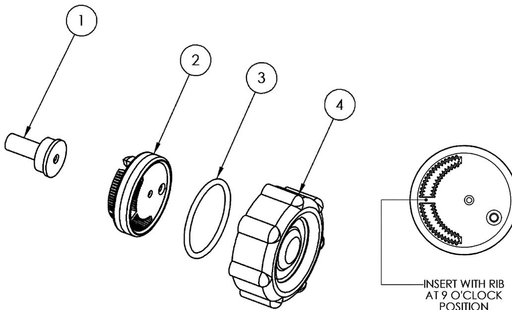
Figure 19: Injector Assembly
