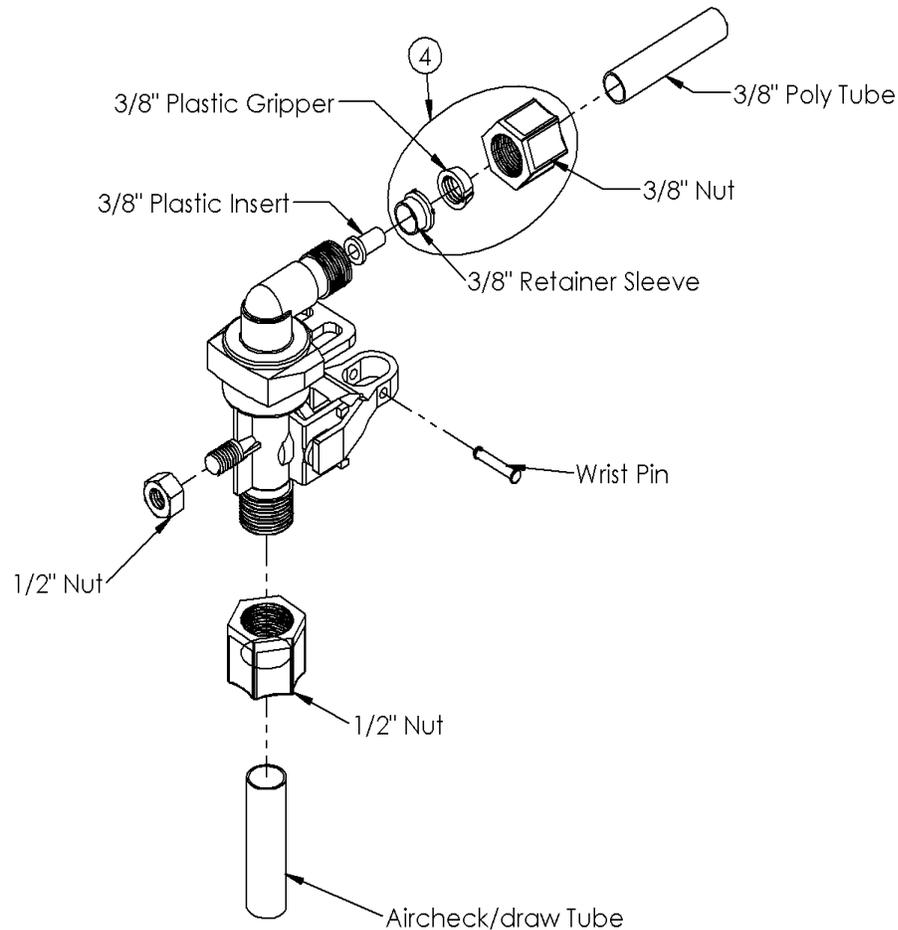
**Figure 23: Brine Valve Elbow Installation**
