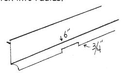
3. Cut two pieces of CactusBoard long enough to allow water to drain past the end of the footing.
